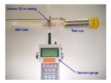
Figure 1. Overview of the test set-up: Sensor casing at the end of the teat cup (Test series A) and two measuring needles (Test series B).
