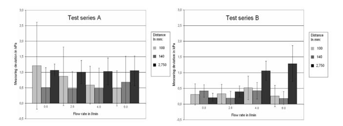
Figure 3. Measuring deviation on the test set-up of test series A and B at different flow rates and at different distances to the teat cup.
