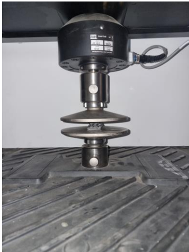
Figure 10. The specimen is under compressive loading.
