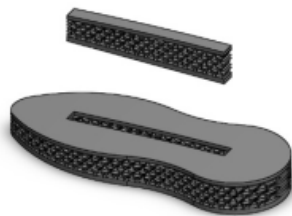
Figure 7. The re-entrant unit cell using ASTM D790 (standard testing method for Bending properties of PTU composite).
