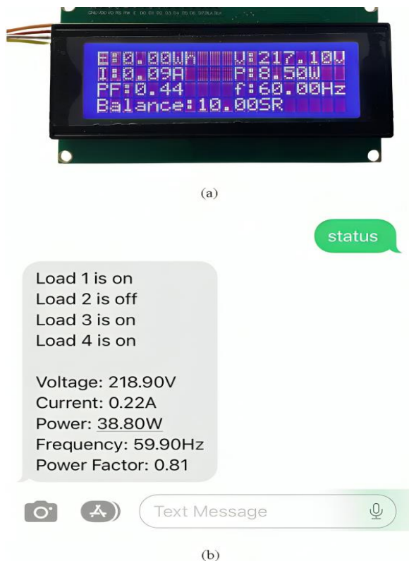
Fig. 5. (a) Power factor and frequency readings on the LCD, and (b) power factor and frequency readings as an SMS message.
