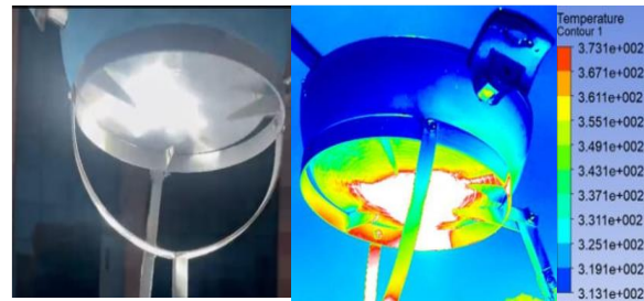
Fig. 4. Temperature contour under cooking pot
