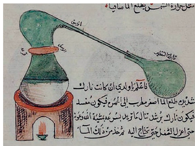
Figure 2. Jabir bin Hayyan described distillation using “alembic” in 8th century
