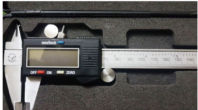
Figure 1. Vernier Calipers used to measure the distances.
