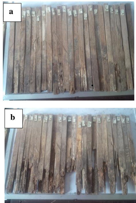
Plate 2.2: (a) Bamboo test samples after six months of Ground contact test in Timber graveyard (b) Bamboo test samples after 12 months of Ground contact test in Timber graveyard.
