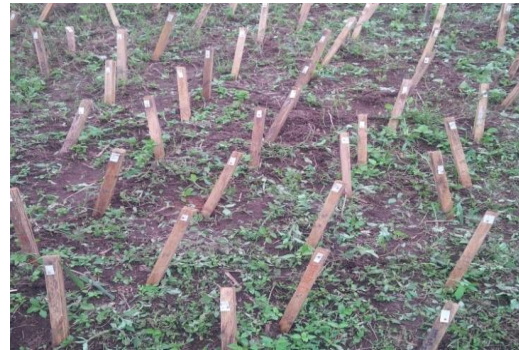
Plate 2.1: Thermally modified and untreated bamboo stakes on the field for Ground contact test in Timber graveyard.
