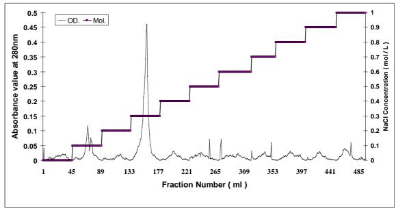
Fig. 11. Final purification of bST on anion exchange chromatography using DEAE-sepharose column. The peaks represent the elution profile of Ion-exchange chromatography conditions: DEAE sepharose with Linear Salt Gradient (0.0-1M NaCI).
