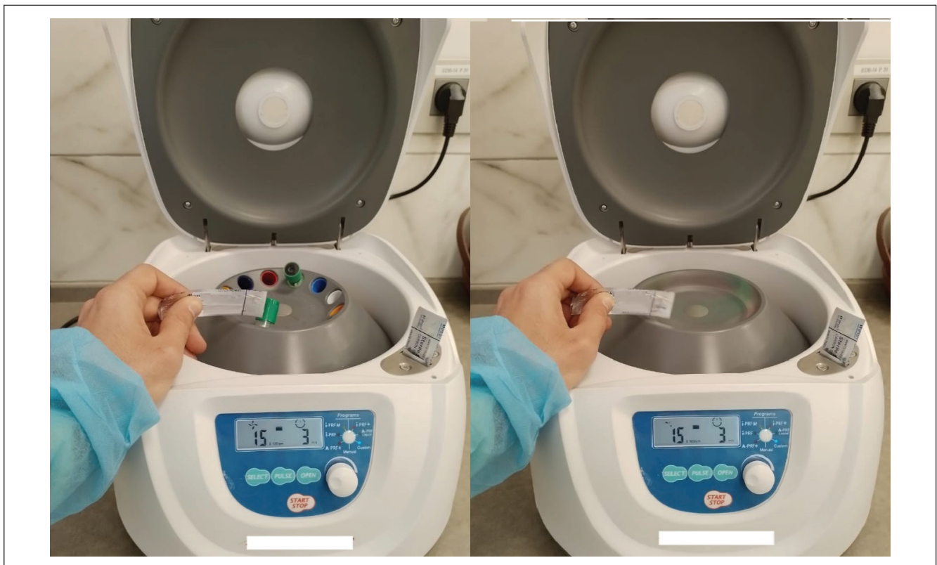
Figure 2. Placement of a thin plastic piece touching the cap of the tubes during their rotation.
