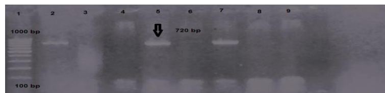
Figure (3): Agarose gel electrophoresis (1.5 %) of the amplified phoA gene of the isolated E. coli . Lane (1): DNA molecular weight ladder (100bp ladder). Lane (2): control positive for phoA gene. Lanes (5, 6 and 7): Positive results for phoA gene (specific band of 720bp). Lanes (3, 4, 8 and 9): negative results for phoA gene.
