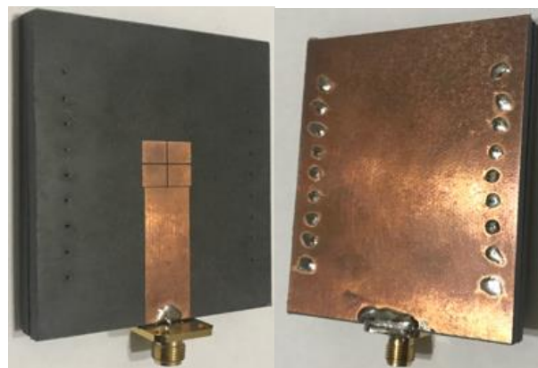
Figure 4. The fabricated 2x2 array LWA with mushroom ground (top view (left) and bottom view (right)).
