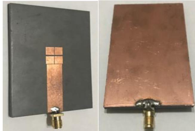
Figure 2. Fabrication of the proposed 2x2 array LWA (top view (left) and bottom view (right)).
